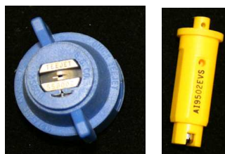
Figure 1. Images showing spray nozzles used in the study. Left, hydraulic Teejet® 8002, Right, Air Induction Teejet® AI9502EVS.
