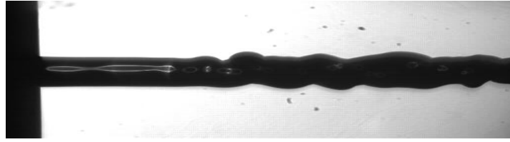
Figure 2. Visualizations of surface deformation of a free jet at Re_i = 3000 [3]
