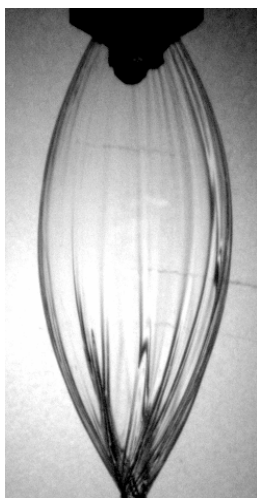
Fig. 3 Closed water bell ( We<35 ).
