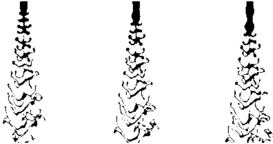
Fig. 4 Water jet into air at Re=10^4 ; We=2219 ; D=400\mu m ; \rho_L/\rho_G=816 ; U_0=28.42m/s .
