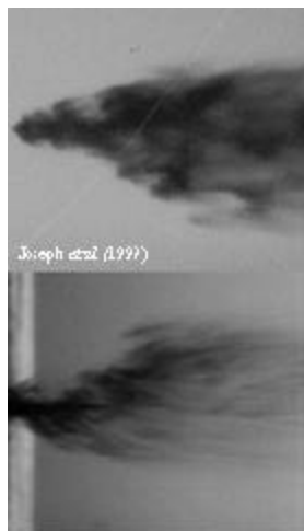
Figure 7 - Instantaneous flow image comparison of the catastrophic breakup of a 2.5 mm water droplet (Joseph et al. [9]) and a 1.0 mm water jet at high Weber number
