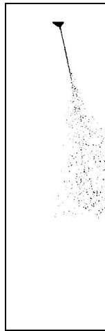
Fig. 2 Typical image of the Taylor cone-jet taken at liquid flow rate of 10 cc/h for an applied voltage of 3.3 kV.
