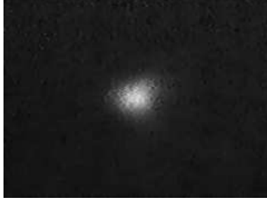
Fig. 6. Light scattered by a droplet, which has entered a region close to the surface, where the evanescent waves are strong enough. The picture shows the scattered light from the same droplet, at the same time, as the droplet, which has produced the shadow shown in Fig. 4. The observed pattern is different from the pattern in Fig. 4 because the scattered light is refracted by the droplet liquid. Corresponding to the shadow the scattered light disappears during the spreading of the droplet.
