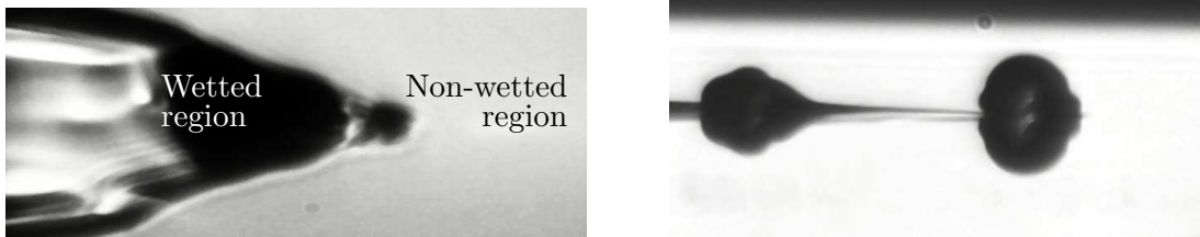
Fig. 3. Images of camera A on the left and of camera B on the right hand side. On the picture on the left the wetted region of the prism surface clearly can be detected. On the picture on the right the corresponding droplets of the droplet stream moving from right to left can be seen forming a liquid film on the prism surface.
