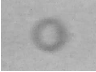
Fig. 4. Circular ring shaped shadow observed in the totally reflected light by camera A. The shadow corresponds to the impingement of a droplet.
