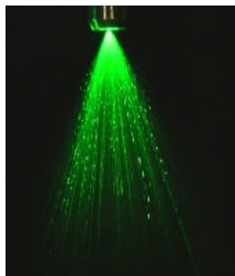
Figure 8. Visualisation of spray of the TG03 injectors
