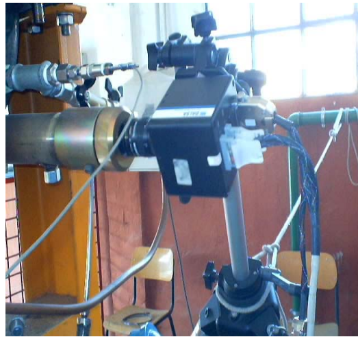
Fig. 2 Lateral/retro view of the LRPM and particular about camera and pressure sensor positions.
