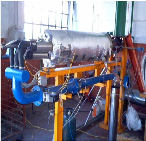
Fig. 2 Lateral/retro view of the LRPM and particular about camera and pressure sensor positions.
