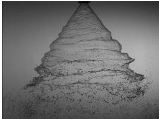
Figure 1 – Spray produced by the pressure swirl atomizer
