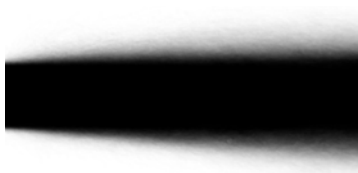
(a) : 20 MPa, delay time = 605 \mu s (maximum needle lift)
