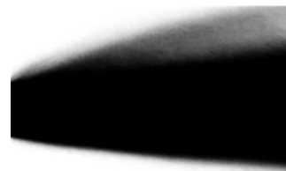
(b) : 60 MPa, delay time = 845 \mu s (maximum needle lift)
