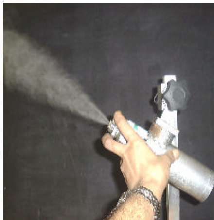
Figure 9: Multi exits and multi throttle models for air fresheners with reduced VOC.
