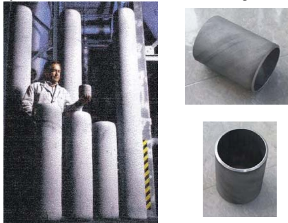
Fig. 1: Spray formed billet and a cylinder liner made from a spray formed billet (PEAK Werkstoff GmbH)
