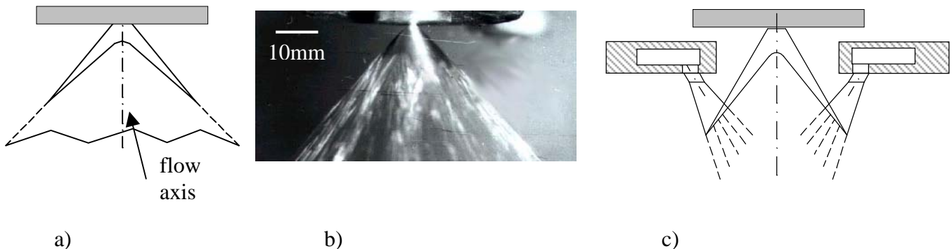
Fig. 1: Schematic of CHA, cross section of the conical film (a), picture of CHA with tin alloy (b), schematic of new atomization technique (c)
